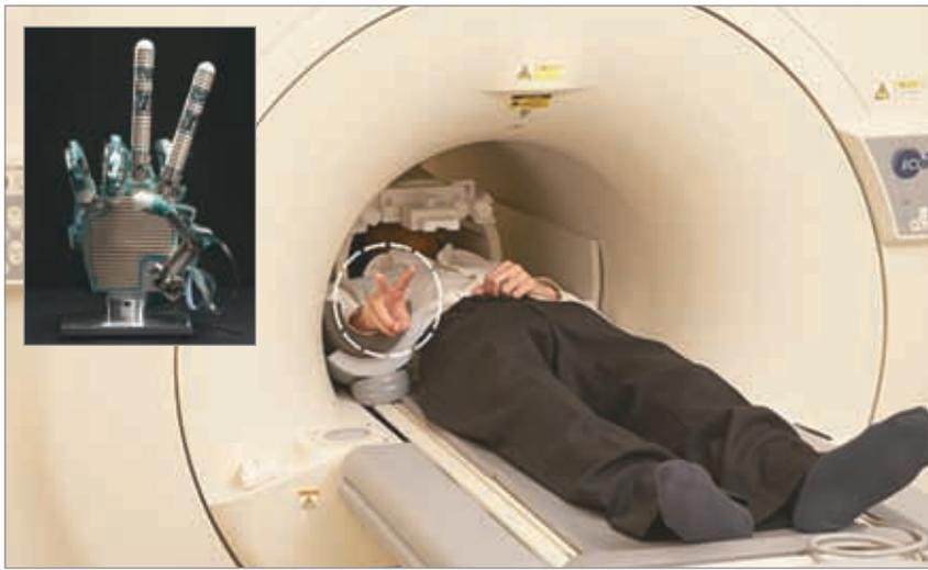
*Figure 1. Honda Motor Corp. has developed a BCI system that can operate a robotic hand. When a subject moves a hand or fingers, the system's MRI scanner detects the brain signals, processes them, and uses software to command a robotic hand to move the same way.*
